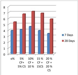
Figure 6. Flexural test results of concrete beam for 7, 28 days
