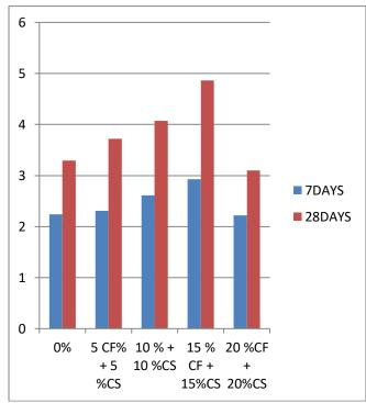
Figure 5. Graph shows the Tensile strength of cubes after 7, 28 days
