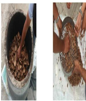
Figure 3. Breaking & sieving of coconut shells to required size.
